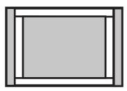
The insides are framed with 2"x2" to offer rigidity. Note the boards for the sides are inset to receive the front and rear panels.
