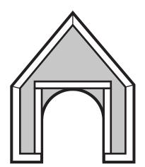
Additional 2"x2" framing around the inside of the dog door. The door is 22" tall & 18.375" wide
