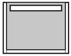
Underside of roof has 2"x2" edging for rigidity. Near the top is a 2x4 for mounting hinges that allow the roof to fold flat. The 2x4 is sized so it seats between the peaks of the front and rear thus locking it inposition.
