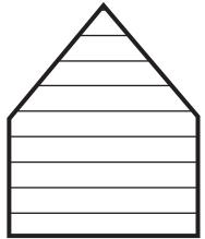
Front & Rear = 47.25" x 38.75" The angle begins 24" up from the bottom. (Two are required)
