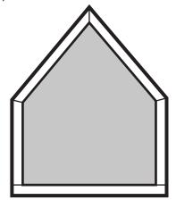
The front and rear have 2"x2" edging for rigidity inside. The two vertical strips are used when screwing the side to the front and rear panels.
